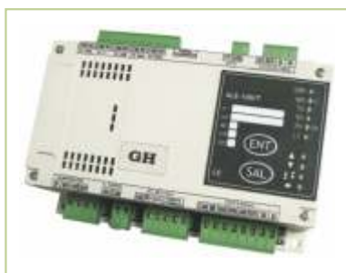
Electronic load limit device (ALE-100/TN)
